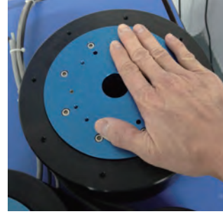
Rotate motor by hand to feel cogging effect
