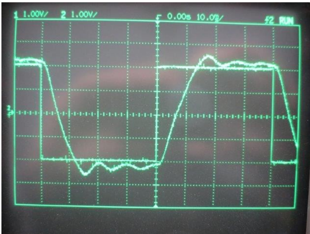
Figure 91: D-Gain too small: Oscillations.
