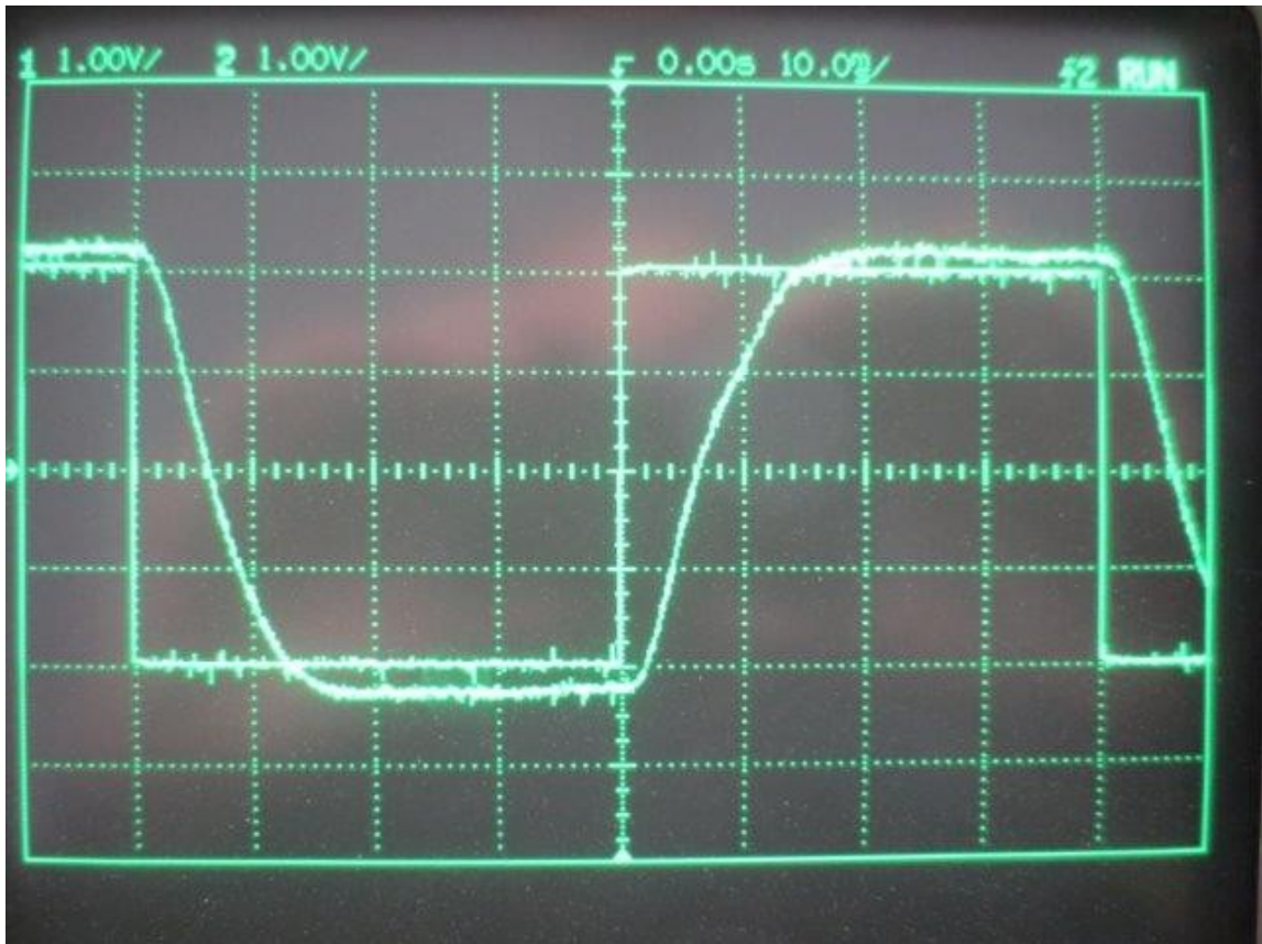
Figure 89: Reference Waveform of perfect adjusted Speed Controller
