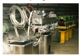
The LHC collimation system (over 150 individual collimators are situated around the LHC ring) protects the accelerator against such beam loss; which would otherwise impinge the supramagnets and cause them to fail ("go critical"). http://lhc-collimation-project.web.cern.ch/lhc-collimation-project/
