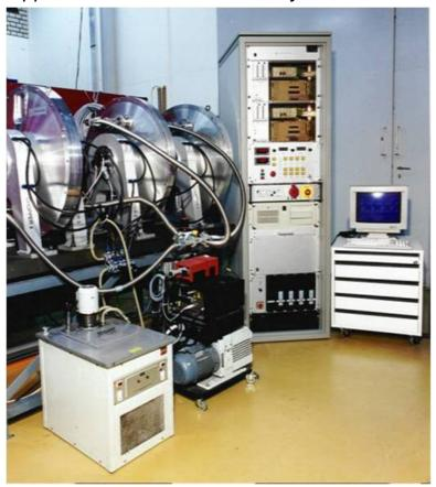
In the field of semiconductor research atomic particle sources are needed with defined particle speeds and thus energy levels (E=mc²). These sources are mounted next to atomic research reactors, which produce a wide spectrum of subatomic particles of different masses and energy levels. A mechanical chopper system is used to select particles within a narrow energy band, by allowing only those particles to pass, which are travelling at a very closely defined speed.
