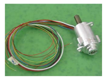
The prototype valve actuators are driven and positioned by the SWM controller under CANbus communication
