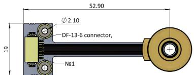
Encoder with flexible connector bus (bottom view).
