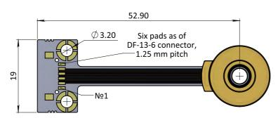
Encoder with flexible connector bus (bottom view).
