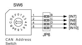
Note: To use inputs 7,8,9, or 10 as logic inputs remove jumpers shown at left to disconnect SW6 from logic inputs.
