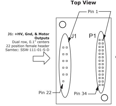
**Drive viewed from above looking down on the pc board on which it is mounted.**Pins shown in grey are unused locations in PC
