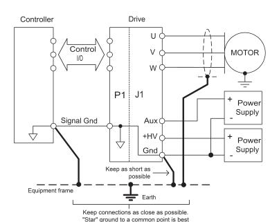
the motor phases, and motor shield currents circulating between the U, V, and W outputs and HV common. And, lastly, logic and signal currents connected to the drive control inputs and outputs. For CE compliance drive cables should be shielded. Motor phase currents are balanced, but currents can flow between the PWM outputs, and the motor cable shield.
