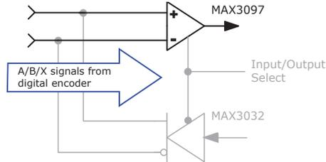
**CURRENT or VELOCITY COMMAND INPUTS: DIFFERENTIAL**
