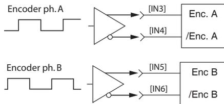
DIGITAL COMMAND INPUTS: VELOCITY, TORQUE
