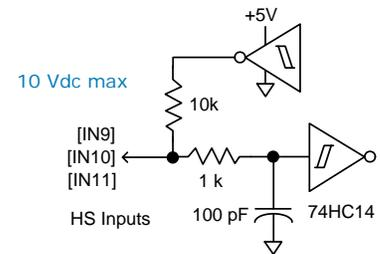
HSD (HIGH SPEED DIFFERENTIAL) DIGITAL INPUTS
