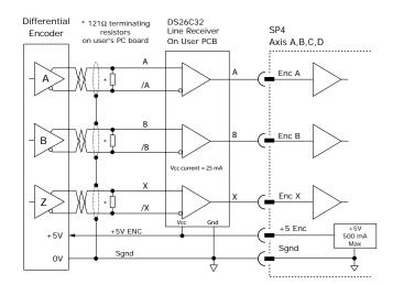
This graphic shows both encoder and line-receiver powered from the SP4 +5V output. If four encoders are connected like this, and assuming 25 mA for each line-receiver, then the available +5V power for each encoder would be 100 mA.
