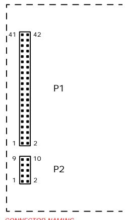
CONNECTOR NAMING (P1, P2, ETC) APPLIES TO THE SP4 MODULE AND NOT TO PC BOARD MOUNTED SOCKETS
