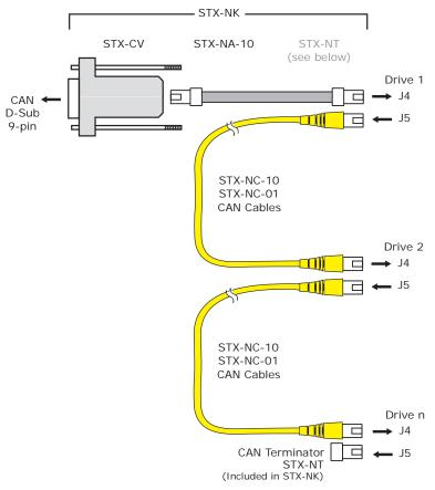
The connector kit for CAN networking (STX-NK) provides the parts to connect to a single drive. These comprise the adapter that converts the CAN D-Sub 9 connection to an RJ-45 type, a 10 ft (3m) modular cable, and a termimator that plug into an RJ-45 socket. The CAN address of the drive must between 1 and 127.
