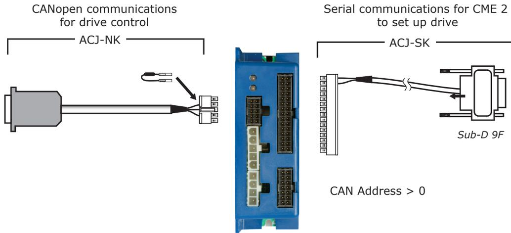
When using CME2, the CAN bus communications should be suspended.
