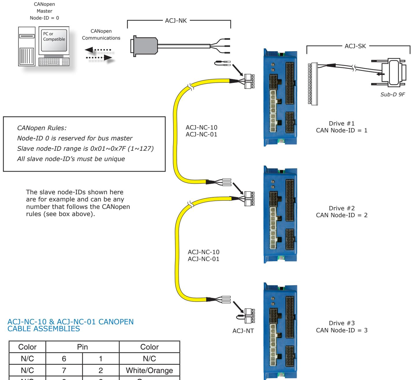
These cables connect to amplifier J1 and have 3 conductors of AWG 24 wire that are terminated in contacts that can then be inserted into pins 7~9 of another ACJ-NC-10 to "daisy chain" the CAN signals to multiple amplifiers.
