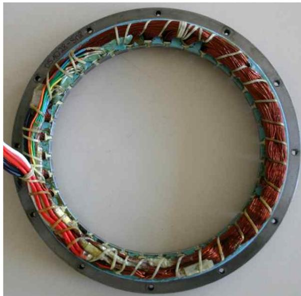
**Stator of MF-motor with axial mounting holes**
