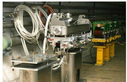
The LHC collimation system (over 150 individual collimators are situated around the LHC ring) protects the accelerator against such beam loss; which would otherwise impinge the supramagnets and cause them to fail ("go critical"). <http://lhc-collimation-project.web.cern.ch/lhc-collimation-project/>
