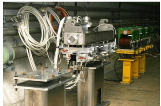
The LHC collimation system (over 150 individual collimators are situated around the LHC ring) protects the accelerator against such beam loss; which would otherwise impinge the supermagnets and cause them to fail ("go critical"). <http://lhc-collimation-project.web.cern.ch/lhc-collimation-project/>
