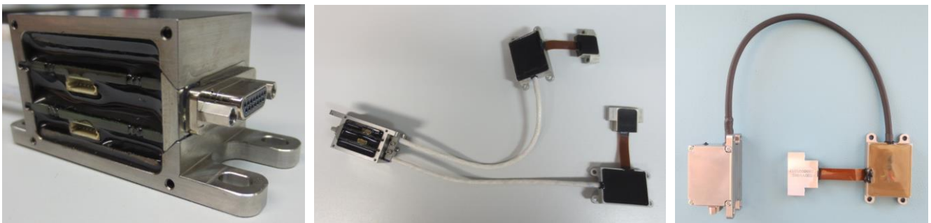
Figure 4. Signal Conversion Box (open, showing configuration interfaces) [left side] Converter Box with interface box to reading heads, [center and right]
