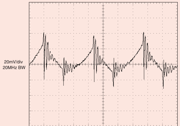
UWR-5/8-D24A Output Ripple and Noise (PARD) (V IN = 24V, full load, external 0.47μF output capacitor.)
