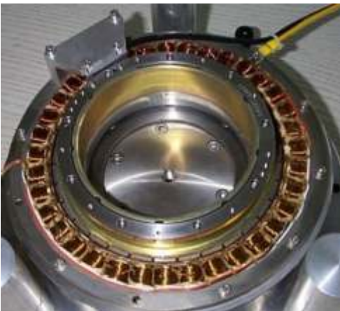
BLDC inner-rotor motor with a high resolution encoder and integrated bearings
