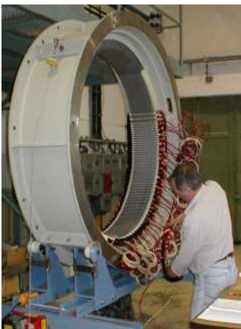
Winding a torque-motor stator
