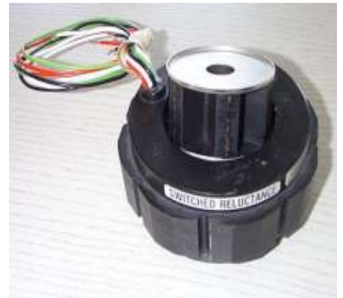
4 phase SR-motor for EMA truck brake system
