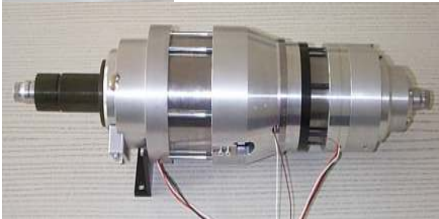
"Steer-by-wire" actuator with two torque motors
