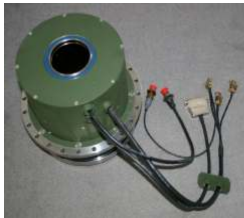
Hollow shaft motor with Harmonic Drive gearbox for pedestal positioning
