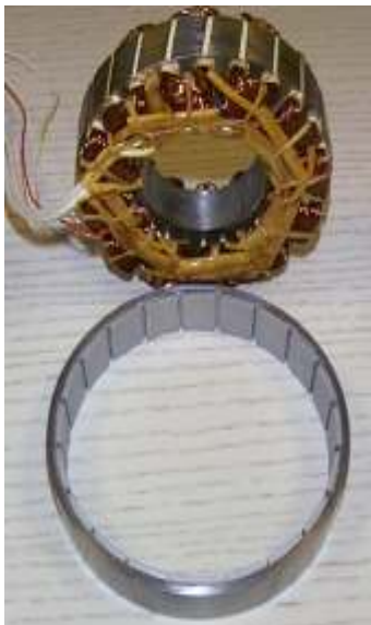
Outer rotor motor for a steer-by-wire actuator
